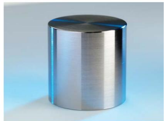
▲ Figure 2 The international prototype kilogram.
