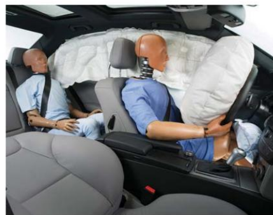
▲ Figure 12 Car safety: seat belts and air bags.
